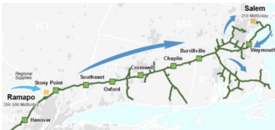
Image 1: Map of the AGT pipeline and compressor stations (square boxes) along the route.
